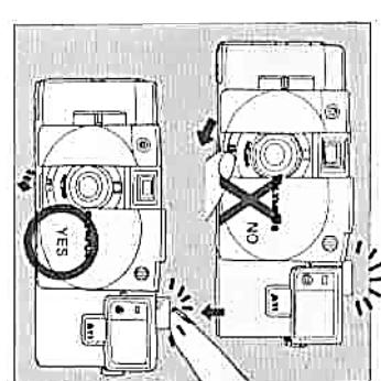
The long-exposure warning signal goes out after 90 seconds. It turns on again when the Dust Barrier is closed and opened.
